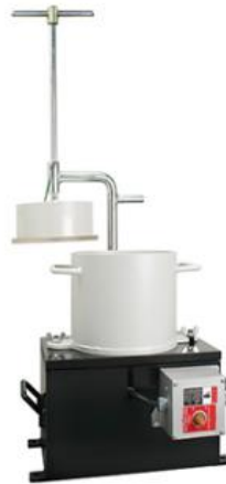
Figure 12. VB apparatus used for experimental packing test
